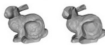
Figure 3: A detailed bunny and one simplified by 98%. From far away the difference isn't that obvious. [4]
