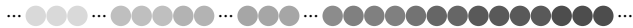
Figure 2: Particles sorted with respect to the cell index. Particles that share the same cell are adjacent in this list.
