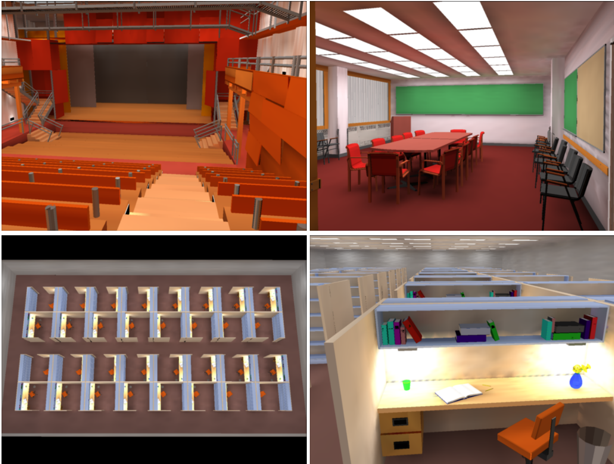
Figure 12: Complex scenes rendered with hierarchical Monte Carlo radiosity: theater (39,000 initial polygons, refined into 88,000 elements, 5 minutes), conference room (125,000 polygons, refinement yields 178,000 elements, 9 minutes) and cubicle office space (128,000 polygons, refined into 506,000 elements, 10 minutes).
