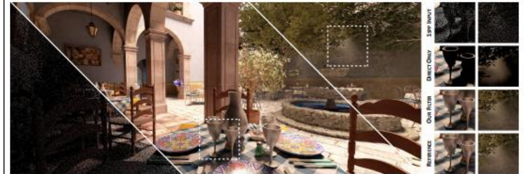
Figure 1: Our filter takes (left) 1 sample per pixel path-traced input and (center) reconstructs a temporally stable 1920 \times 1080 image in just 10 ms. Compare to (right) a 2048 samples per pixel path-traced reference. Insets compare our input, our filtered results, and a reference on two regions, and show the impact filtered global illumination has over just direct illumination. Given the noisy input, notice the similarity to the reference for glossy reflections, global illumination, and direct soft shadows.
