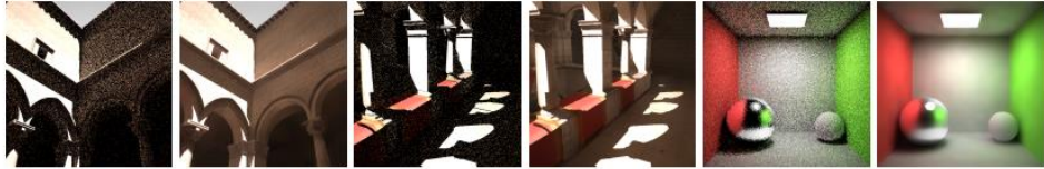
Figure 1: Using our edge-avoiding \tilde{A} -Trous wavelet transform we filter highly noisy path traced images at interactive rates resulting in smooth indirect illumination while retaining important detail like sharp shadows and hard edges. The images show the (noisy) input into our algorithm and next to them the output we compute.
