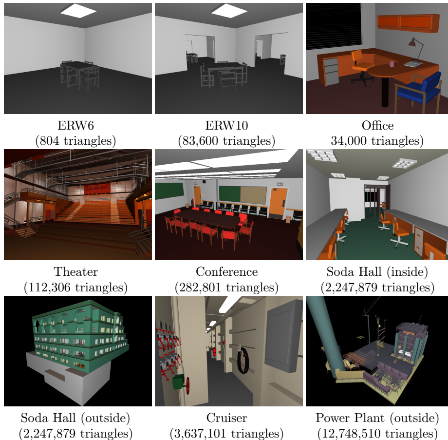
Figure 7: The scenes used for the RTRT benchmarks in Table 6. Including simple SSE shading, these scenes run at 1.3–5.4 frames per second at full-screen ( 1024 \times 1024 ) resolutions on a single 2.5GHz Pentium-IV notebook CPU.
