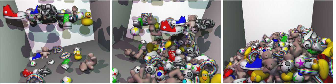
Figure 9: In this massive scene consisting of 384 objects, the computation of the dynamics is possible in real-time while collision detection and collision response computations are not.
