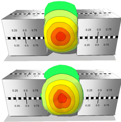
Figure 8: A soft sphere is squeezed between two stiff cubes. The purpose of this experiment is to illustrate the behavior of the collision response scheme at high pressures. Top: Collision response by computing the contact surfaces. Bottom: Collision response using a penalty-based approach. Note the significant overlaps of the sphere and the cubes in the resting state.
