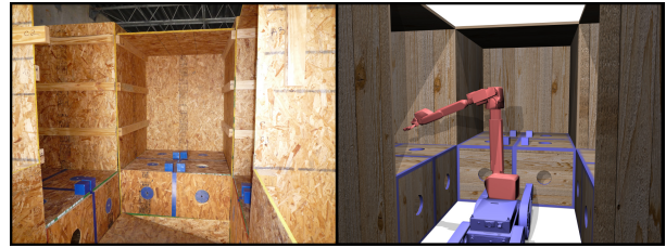
Fig. 1. The manipulator dexterity test. Left: Original setup as used in Disaster City. Note the horizontal bars that can be used to mount vertical boards extremely restricting the robot’s workspace. Right: The reconstruction we use in our experiments.
