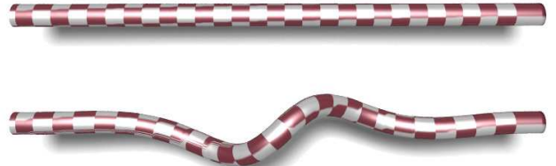
Fig. 5. A perfectly straight rod that is subject to a torsional load is in an unstable equilibrium (top). As soon as the centerline is slightly disturbed, the rod starts to bend until an equilibrium between torsion, bending and stretching strain is reached (bottom). Approaches that do not treat bending and torsion in a unified manner cannot reproduce this behavior. This experiment provides a simple way to verify the physical plausibility of an elastic rod deformation model.
