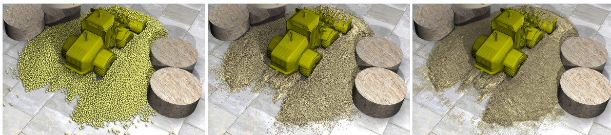
Figure 1: The proposed framework simulates mechanical behavior at a coarse scale (left). The base simulation is significantly refined with a secondary simulation (middle and right). Simulation particles (38K, 1.4M and 19.4M, left to right) are rendered.
