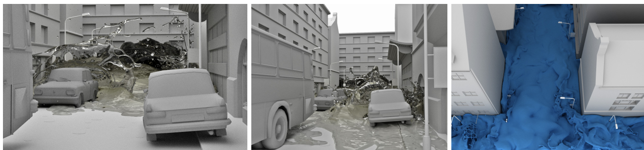
Fig. 11. Street flood. This scene contains up to 28 million fluid particles. IISPH computes one simulation step in 42 seconds with an average time step of 0.0025 seconds and a compression of less than 0.1%.
