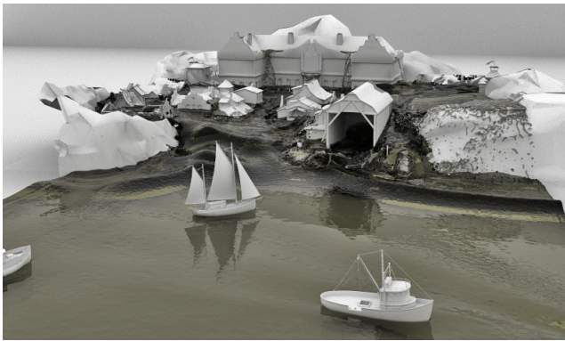
Fig. 10. A scripted island rises out of the water. 10 million SPH fluid particles. One simulation step is computed in 14 seconds with a time step of 0.0054 seconds and a compression of less than 0.1%.
