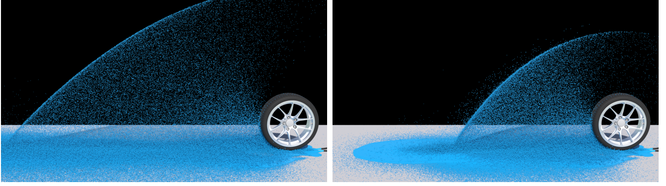
Figure 2: A wheel rotating with a speed corresponding to 20\text{kmh}^{-1} . When not using our drag force (left), the particles are sprayed very far. Applying our drag force (right), the particles reach a terminal velocity and the spray distance matches real-world experiments.
