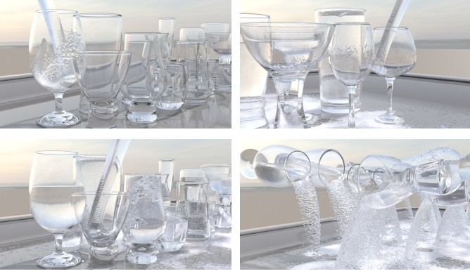
Figure 9: Glasses scenario with various complex boundary shapes and up to 26 million fluid particles simulated with our approach.
