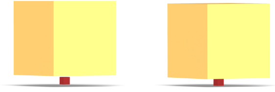
Figure 6: A heavy rigid block (yellow) is dropped on a much lighter block (red) where it then comes to rest. The mass ratio between the blocks is 1000 : 1. Our contact handling method is able to robustly handle this challenging constellation.
