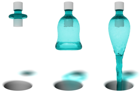
Fig. 8. Two vertical water jets are colliding. Due to surface tension, the water that was initially pushed outwards is pulled together until it merges into a single water stream. The fluid has \gamma^{FV} = 0.16 \text{ N m}^{-1} , the distance between fluid collision and sink is 2 m.
